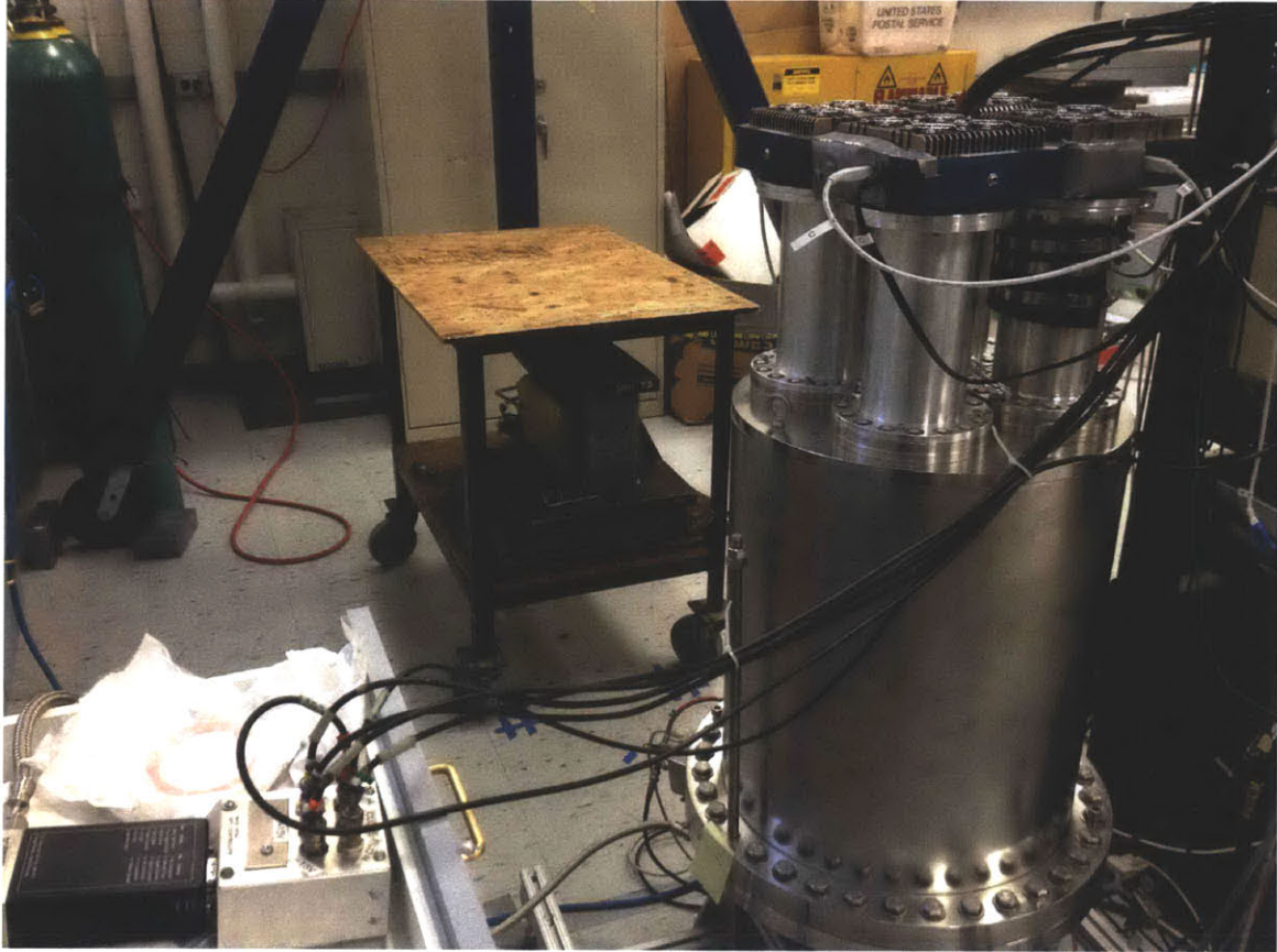
Figure 5-2: A photograph of the Am-Be setup sketched in Figure 5-1. The Am-Be source is in the center of the image, underneath a sheet of RICORAD, and behind a single lead brick, on the cart with wheels. The 4-shooter is on the right in the image, and the edge of the 4-shooter electronics rack is just visible on the far right.
