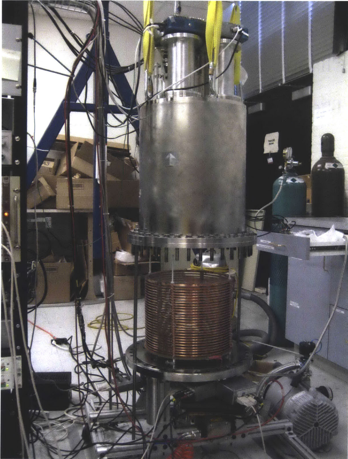
Figure 3-1: An image of the 4-shooter detector in Building 24, Room 036 at MIT. The vacuum vessel is open, showing the TPC. The four blue CCD cameras are visible at the top of the image.
