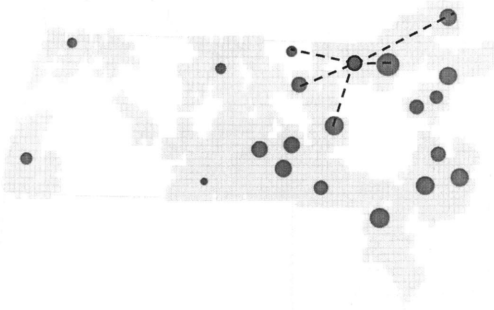
Figure 3.1: This figure demonstrates the method used by the optimization to assign each job to a platform. The amount of time to complete a job from a given platform is represented by the length of the corresponding dashed line. Intuitively, a given repair will take longer if the crew assigned to it is dispatched from a further platform.
