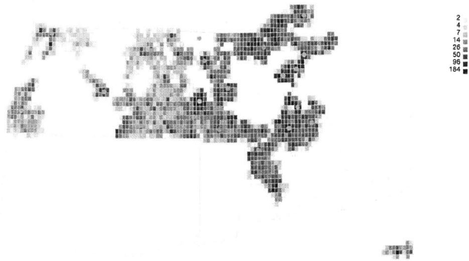
Figure 2.2: This figure illustrates the density of the local distribution electrical network in Massachusetts. The state is partitioned into square areas of 2 miles per side which are colored by the number of assets they contain. In particular, notice that this electricity provider covers most of the rural areas but not the Boston agglomeration. Finally, the orange circles represent the platforms where the company stages repair crews before and during large storms.
