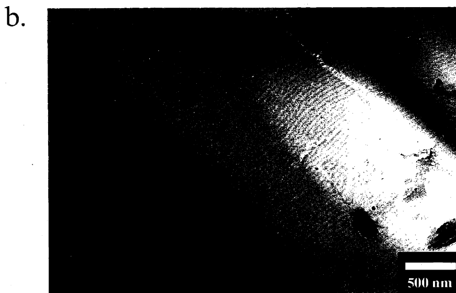
Figure 9.6 TEM bright-field images of a thin film of PS/PI(45/12) block copolymer, directionally solidified with BA, and treated via O 2 -RIE. Void microdomain structure after removal of the PI cylinders by O 2 -RIE appears brighter. (a) Thinner block copolymer film shows vertically ordered cylindrical microdomains to the substrate (b) Thicker block copolymer film shows directionally solidified PI microdomains oriented parallel to the substrate.
