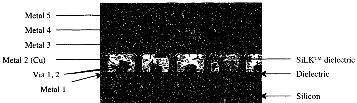
Figure 2.1 Cross-sectioned scanning electron micrograph of SiLK™ dielectric in copper dual damascene integration scheme. (Courtesy of IMEC, Hitachi)
