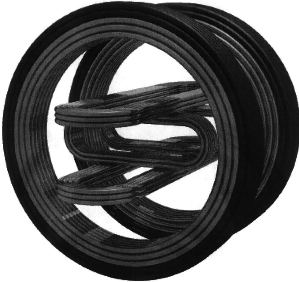
Figure 5.3: Modified Ioffe-Pritchard Trap. In this rendering of our modified IP trap, each of the different coils can be seen. The shorter “racetrack” coils running left and right are the elongated pinch coils. The two long coils above and below the pinch coils make up the gradient producing Ioffe bars. The large round coils are divided into two sections, differentiated by different colored wire. The inner, lighter colored windings make up the “anti-bias” coils, and the darker outer windings make up an extra set of coils which can be used to generate large bias fields if they are required by an experiment. Bias fields produced by these extra coils are also used to weaken radial confinement of the trap (see Section 5.4).
