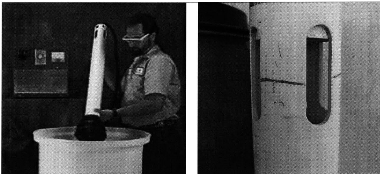
Figure 4.3 – The electrolytic cell and the circulation slots
