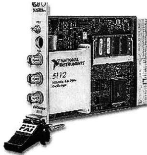
Figure 7: A PXI (PCI eXtensions for Instrumentation) Data Acquisition Card
