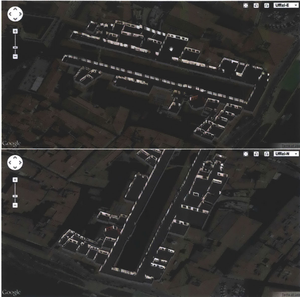
Figure 5-33: A global texture-mapped mesh model allows indoor scene visualization based on pre-rendered tiles, which has been a popular technique for online digital mapping products. We generate tiles for four different headings (i.e., north, south, east and west) in multiple resolution levels by using the view-dependent wall models, where back-facing walls are lowered to improve visibility for each direction. This figure shows the Uffizi Gallery from the two different headings.
