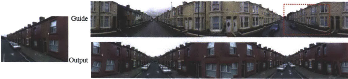
Figure 3-11: Our method can extrapolate an image of limited field of view (left) to a full panoramic image (bottom right) with the guidance of a panorama image of the same scene category (top right). The input image is roughly aligned with the guide image as shown with the dashed red bounding box.
