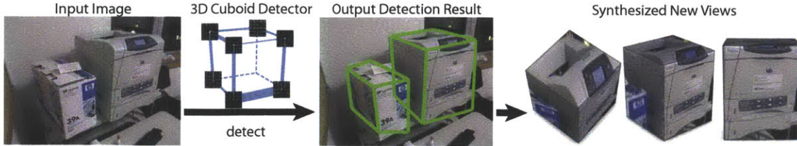
Figure 4-1: Problem summary. Given a single-view input image, our goal is to detect the 2D corner locations of the cuboids depicted in the image. With the output part locations we can subsequently recover information about the camera and 3D shape via camera resectioning.
