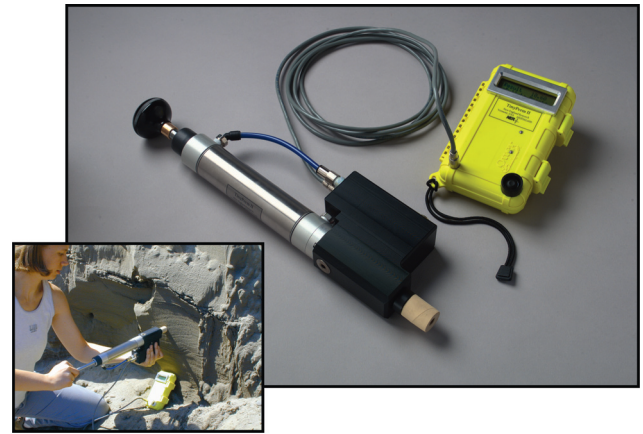
Figure 3. Photographs of the syringe air permeameter.
