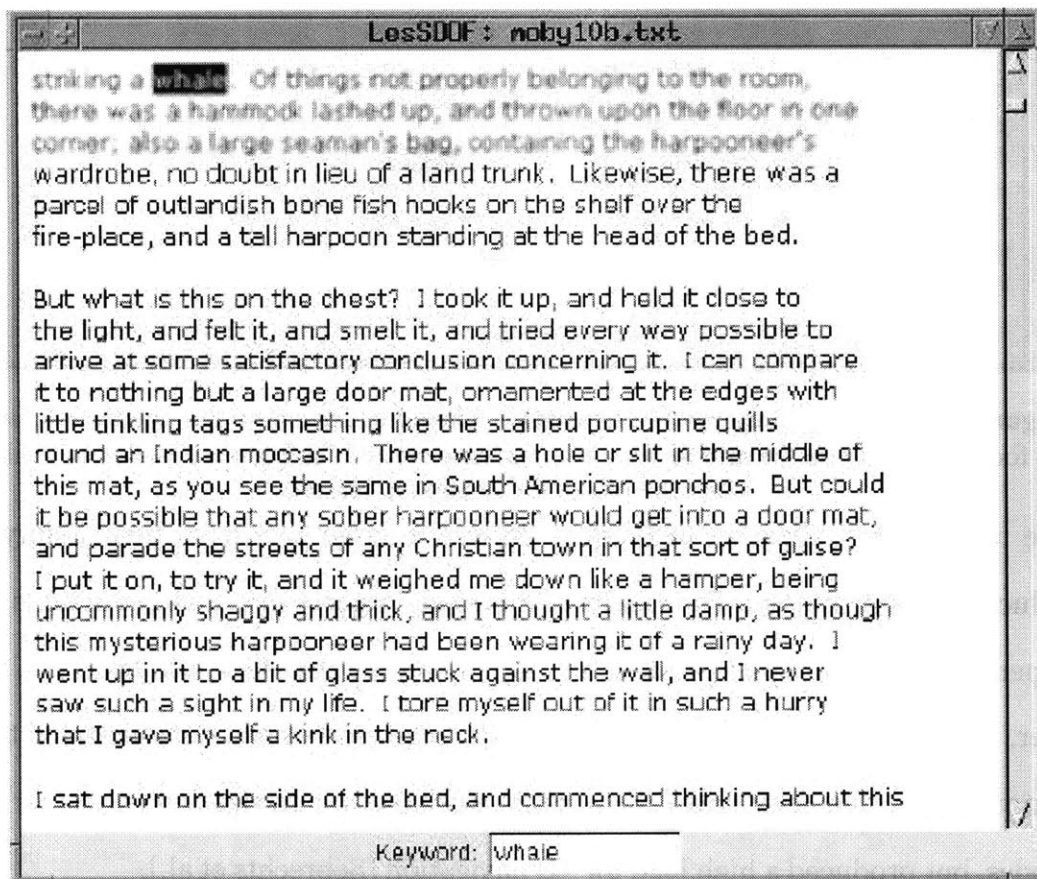
Figure 3.3: Scrolling in LessDOF. Three lines on the top are context from the last page, and therefore blurred, but still readable.
