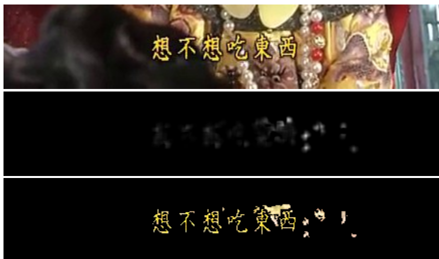
Figure 3.15: Restricting pixels to those that both match the subtitle color and are near corners reduces extraneous artifacts, but does not always eliminate them.
