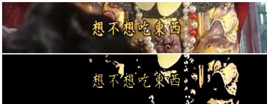
Figure 3.14: Simply extracting out the pixels which match the subtitle color results in an image with extraneous artifacts.
