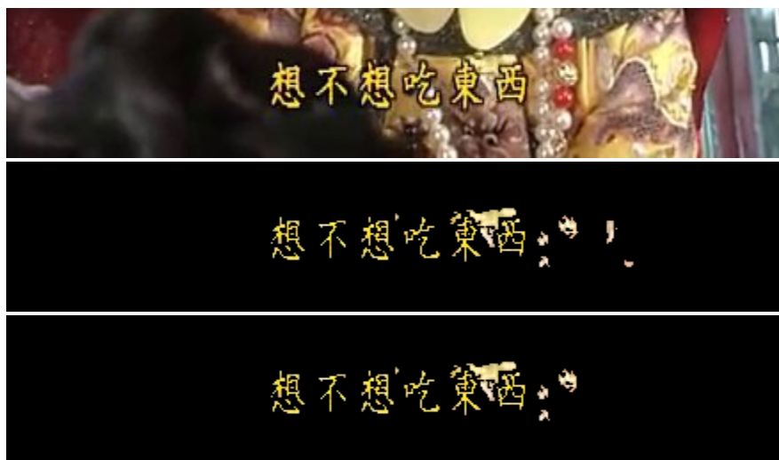
Figure 3.18: Determining the horizontal span of the subtitle further eliminates some extraneous pixels.
