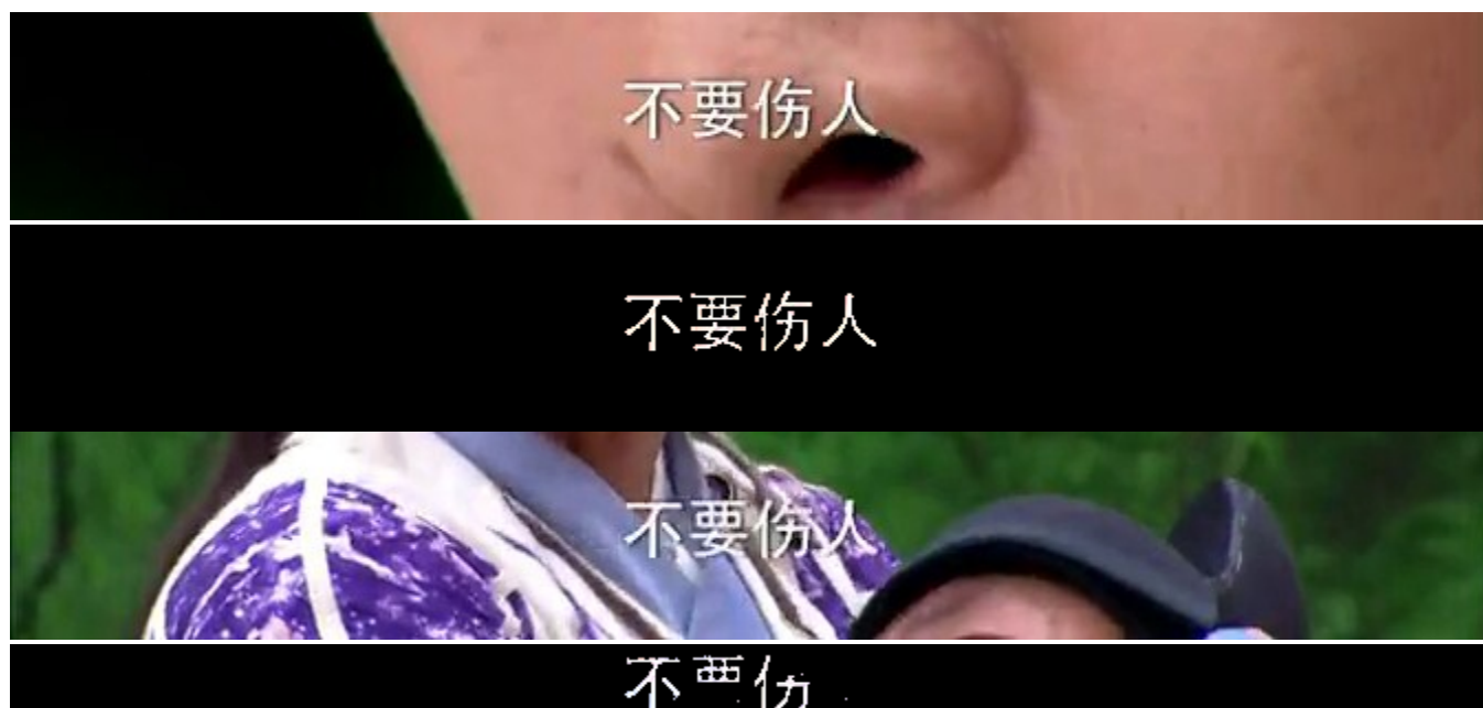
Figure 3.20: This figure illustrates why we should not simply take an intersection over all frames to determine the final set of pixels which we will use for OCR. On the first image, applying our subtitle-isolation heuristics in isolation results in a good set of pixels that can be OCR-ed to obtain the subtitle. However, our subtitle-isolation heuristics perform poorly on a later frame (third image), so simply taking the pixels which are in common across all frames will result in a set of pixels which are unusable for OCR.
