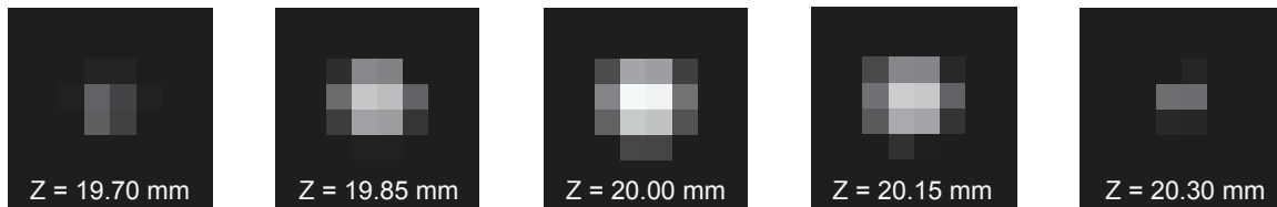
Figure 3-4: Intensity profile of a single synthetic particle refocused using the cost function over focal planes with spacing \delta Z = 0.15 mm. The particle center lies at Z = 20.00 mm. The particle can be represented by a 3D Gaussian kernel in voxel space and localized using this intensity distribution, analogous to a 2D PIV particle image in pixel space.
