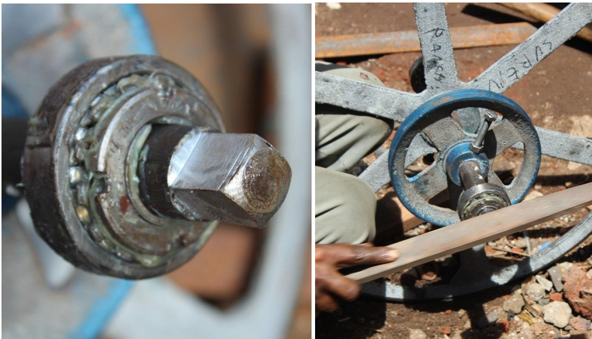
Figure 4.27. Cutting and filing the end of the driveshaft to interface with the handle.
