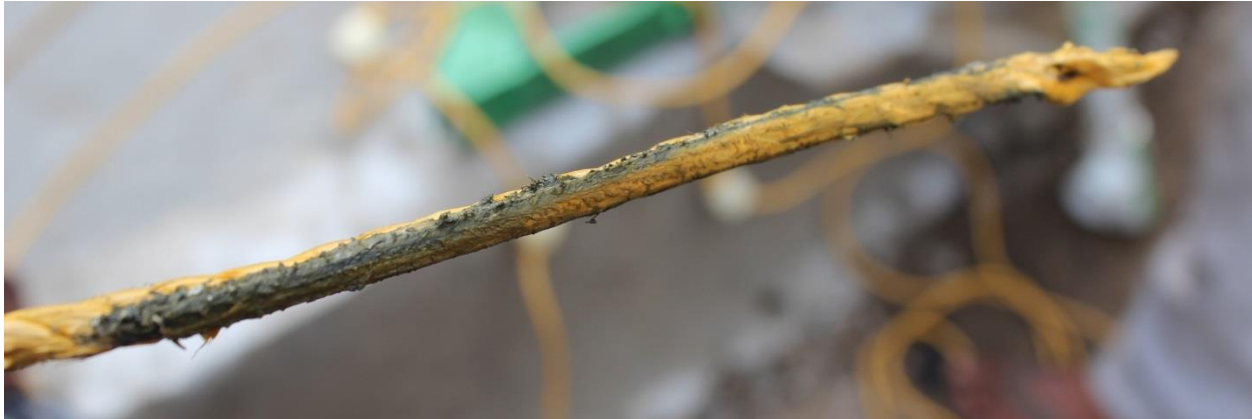
Figure 4.39. Friction on the pulley melted rubber onto the rope and burned it to the point of breaking.
