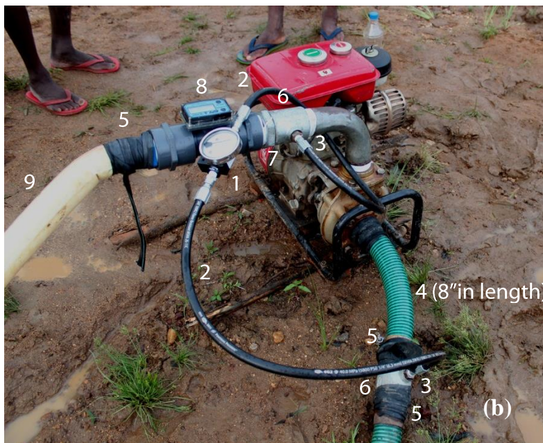
Figure 2.14. Set-up of the pump outfitted with pressure and flow rate instrumentation. (a) Schematic. (b) Photograph. The change in pressure between the pump inlet and the pressure gauge due to the barbs and eight-inch piece of hose are negligible compared to the overall system change in pressure.
