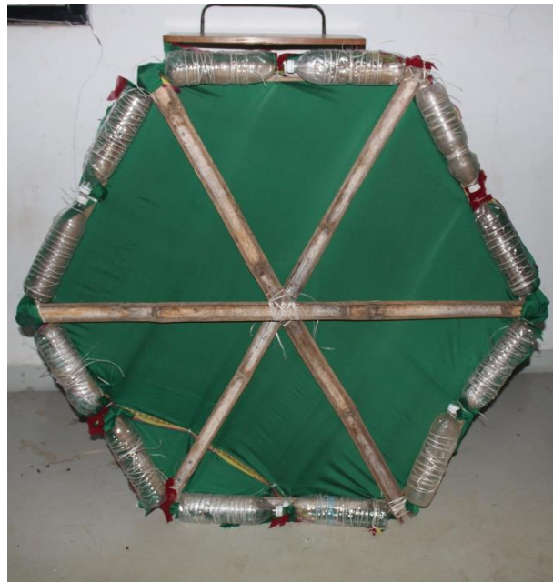
Figure 5.14. Float made of waste PET bottles, bamboo, and old saris.
