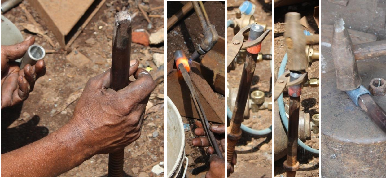
Figure 4.28 Fabricating the part of the hand crank that interfaces with the driveshaft.
