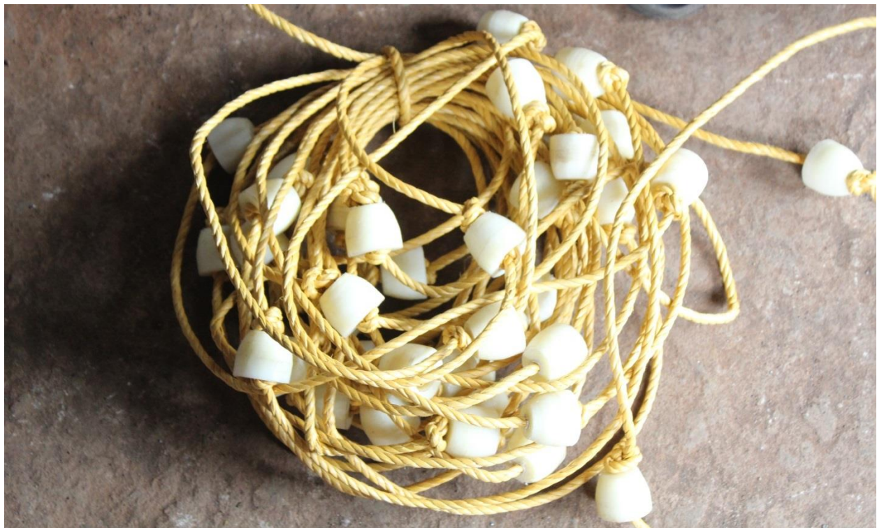
Figure 4.20. Polypropylene (“PP”) rope with nylon pistons.
