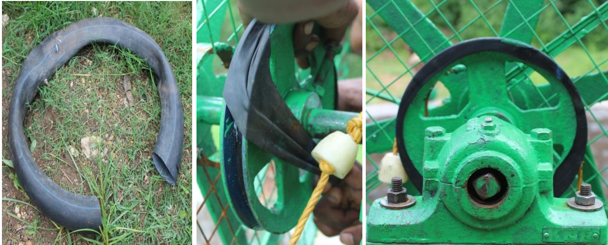
Figure 4.37. A slice of used motorcycle tire was wrapped around the pulley wheel in an attempt to eliminate slipping.
