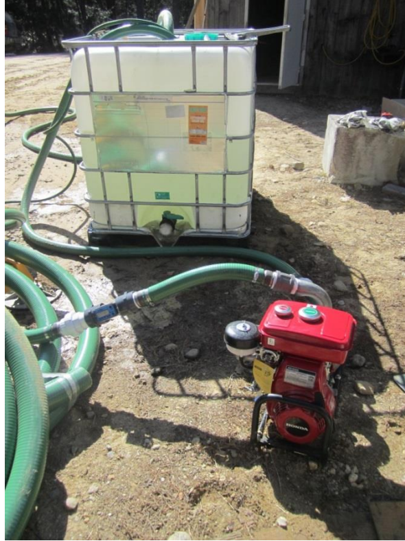
Figure 2.4. A water tank served as the water source for the pump system, and the water level sat above the inlet of the pump during simulated submerged conditions.
