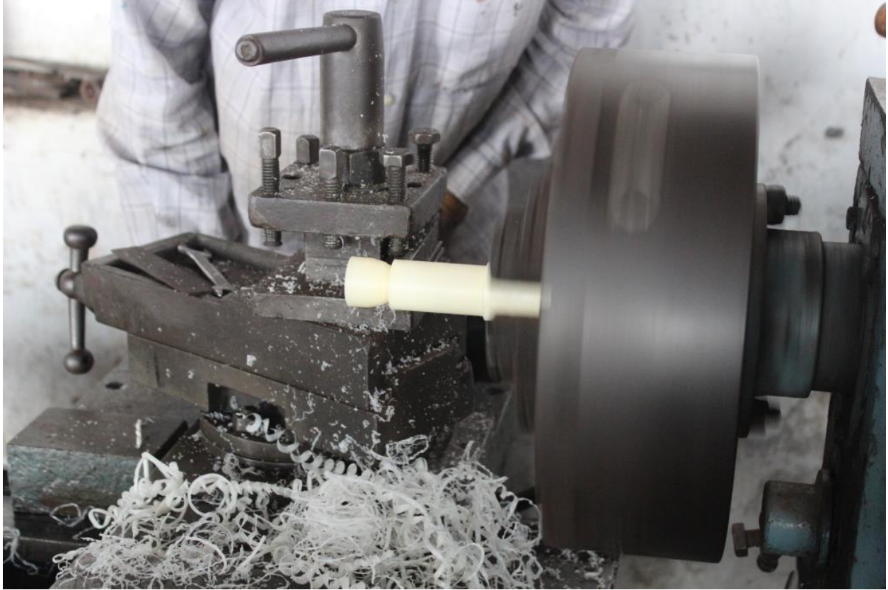
Figure 4.18. Pistons were cut from solid nylon rods on a lathe.
