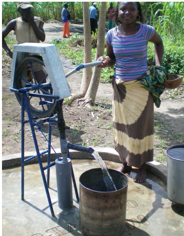
Figure 4.6. Manual rope pump in use in Mozambique. [93]
