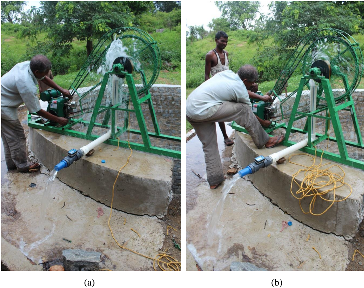
Figure 4.41. Testing the rope pump in engine mode at (a) a higher rpm and (b) a lower rpm. A lot of water is lost through the top of the rising main.
