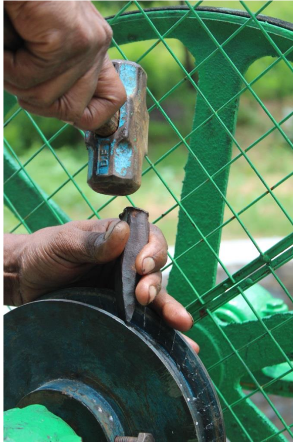
Figure 4.40. Roughening the sides of the pulley with a chisel.
