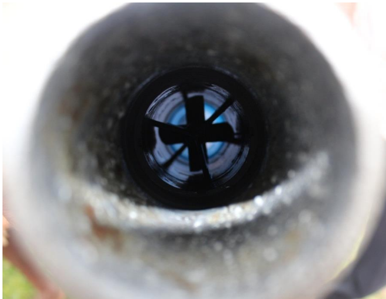
Figure 2.17. The turbine inside the flow meter sometimes got stuck when silt in the water prevented it from turning.
