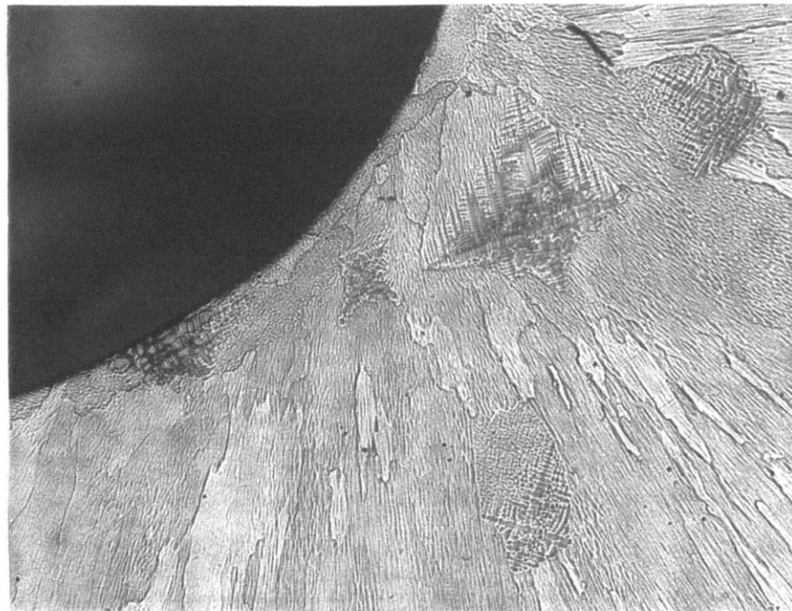
Figure 12 – Microstructure of a high-Ti-alloy specimen melted and gas-cooled in 4%N 2 -gas and then quenched in In-Ga bath after holding at the solidification plateau for 3.5 s: the entire specimen (top) and equiaxed dendrite grains in the frozen core (bottom).
