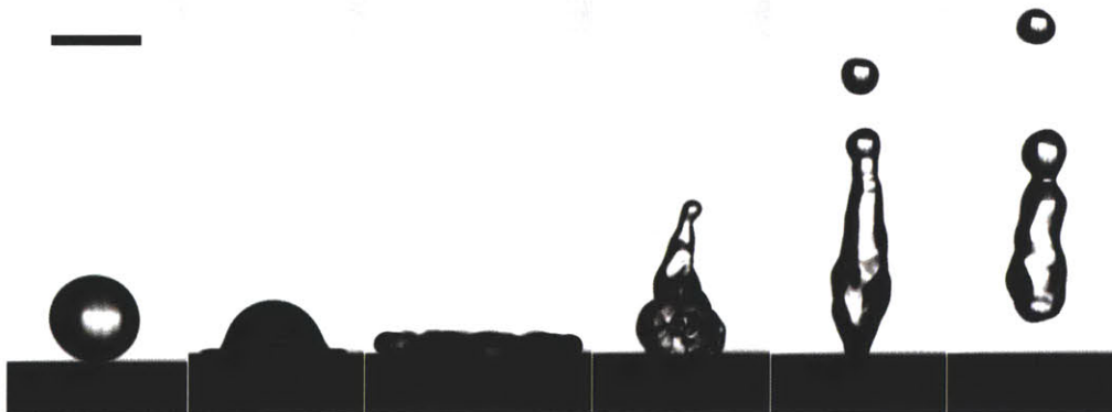
Figure 4-2: Water repellency of laser-ablated ceria sintered pellet. High-speed photography images of a water droplet bouncing off of the laser-ablated ceria sintered ceramic (impact velocity \sim 1.5 m/s); the scale bar is 2.5 mm.
