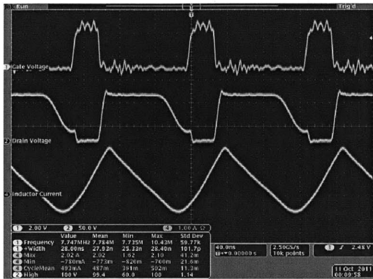
Figure 5-2: Iteration 3 waveforms showing low but nonzero turn-on voltage at 100V in, 35V out
