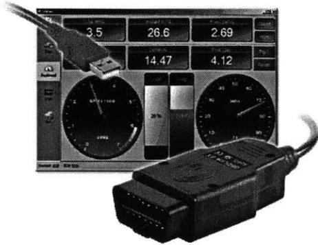
Figure 12: OBDLink SX (source: <http://www.scantool.net/obdlink-sx.html>)
