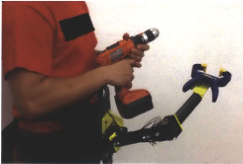
Figure 1-1: Side view of the SRLm prototype, a version of the SRL used for non-physically demanding tasks.
