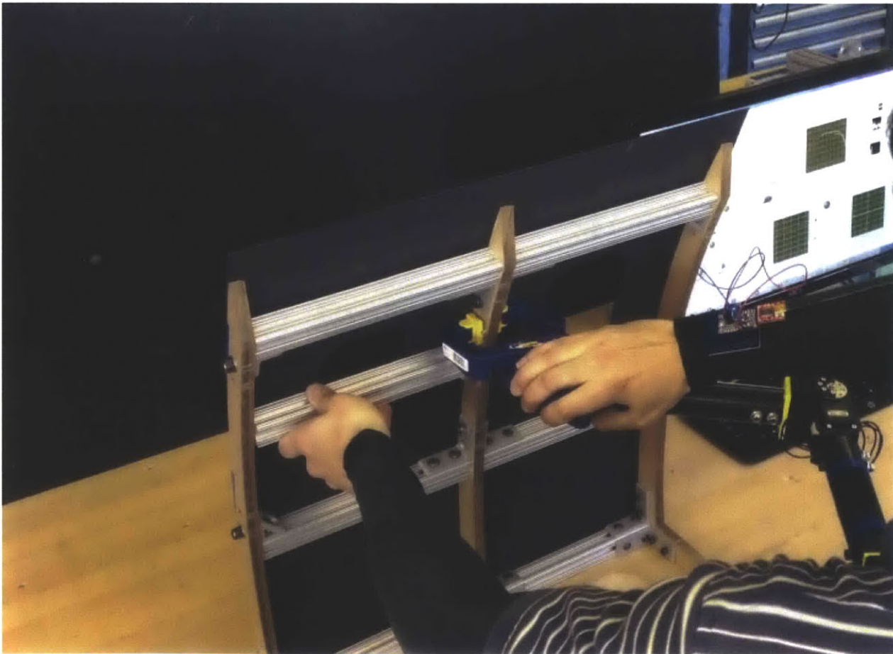
Figure 5-8: Once the operator has positioned the intercostal and given the cue, the SRLm automatically moves in to place the gripper end-effector in its assigned position.
