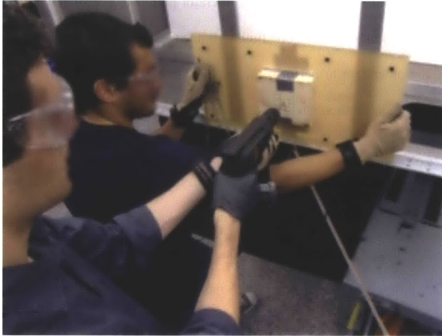
Figure 5-11: Demonstration data acquisition of two workers' cooperative operations: lead worker holds a hand drill while the follower holds a workpiece that needs to be fixed to the plane.
