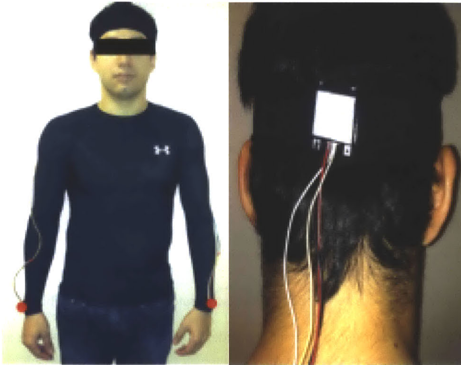
Figure 5-1: The sensor suit has inertial measurement units (IMUs) in the red locations: one on the back of the head and one in each wrist. (a red dot is used in the left picture to locate the IMUs).
