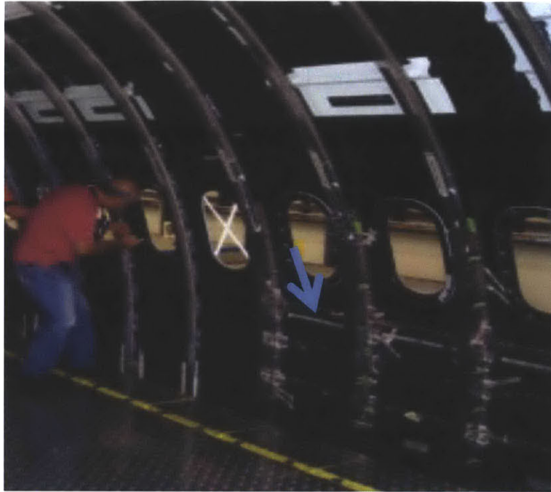
Figure 4-1: The blue arrow points at the intercostals that need to be fixed and drilled into the airplane's fuselage.
