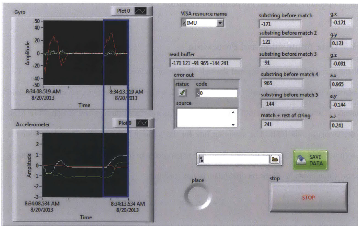
Figure 5-3: Front panel of the VI for acquiring data from the SRLm’s Operator while executing the first transition. The images to the left are the raw data obtained from the IMUs. The circle labeled “place” to the left of the stop button turns on yellow when indicating the operator that he can start performing this sub task. The blue square shows the IMU signals of the right hand during the period in which the SRLM’s operator proceeded to properly place the intercostal.
