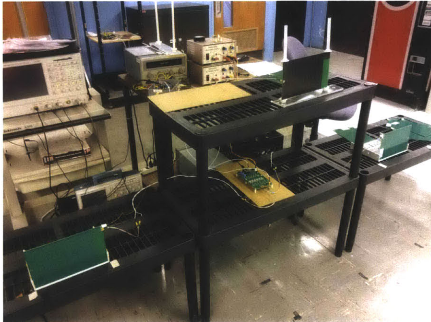
Figure 5-1: Front left view of the standalone sensor setup. The source electrode is located on the highest platform and protected by electrical tape. The receive electrodes are on either side of the source electrode and the sensor board sits between them.
