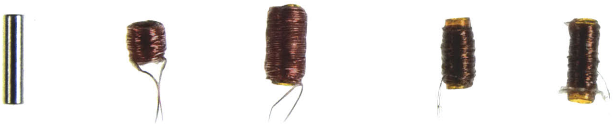
Figure B-2: A collection of experimental coils wound to test various fabrication techniques and examine feasibility. The leftmost two coils were wound with 150 \mu m diameter wire, while the two on the right were wound with 50 \mu m diameter wire. A \phi 1.5 mm permanent magnet is included on the left-hand side for scale.
