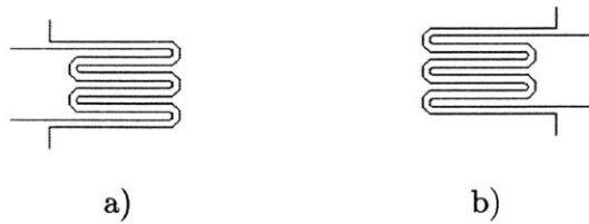
Figure B-2: Closeup of the sensor pattern. a) Design for the sensor on the left (baseline design). b) Design for the sensor on the right (one end supported design).
