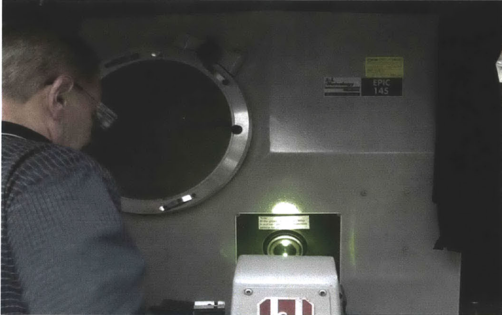
Figure 4.3: Dimension measurements of new micro drill bits
