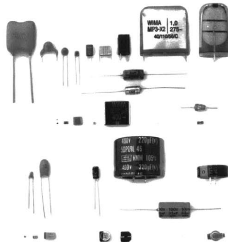
Figure 11: Typical shapes and sizes of capacitors.
