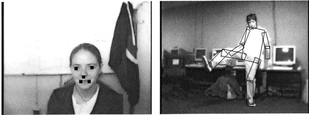
Figure 1-1: Detection results for a face (left) and a human body (right). Each image shows the globally best location for the corresponding object, as computed by our algorithms. The object models were constructed from training examples.
