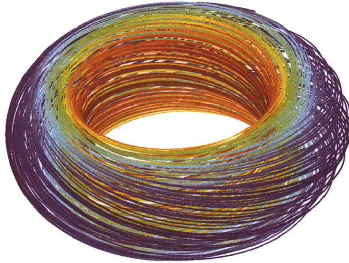
Figure 1-5: Reconstruction of the total magnetic field in Alcator C-Mod for shot 1050426022, t = .64 s. Color indicates field magnitude: Max (red) 7.8 T, Min (blue) 3.2 T.
