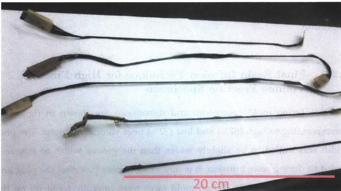
Figure 3.7 Preliminary resin impregnation trials of HTR-40 24K tow. Top sample has a hat-like cross section. Middle three specimens did not achieve full impregnation. Bottom sample was the first successful impregnation by resin infusion through a dry tow situated inside a Teflon channel.
