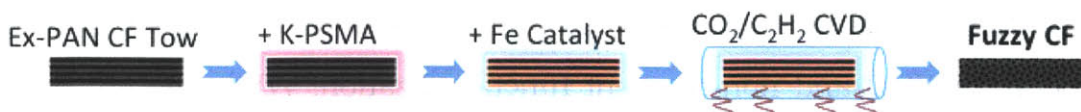
Figure 3.1 Procedure for growing CNTs on CF without degrading filament strength. Ex-PAN fibers are non-covalently functionalized in K-PSMA coating, dip-coated in iron nitrate solution, and subjected to \text{CO}_2/\text{C}_2\text{H}_2 thermal CVD at 480^\circ\text{C} for CNT growth. Resultant tows have circumferential CNT growth around each fiber.
