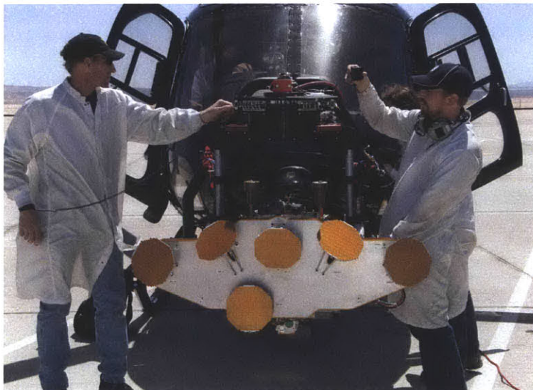
Figure 1-7: Testing an engineering model of the Mars Science Lab Doppler RADAR system, which is used for descent navigation. Image credit: NASA
