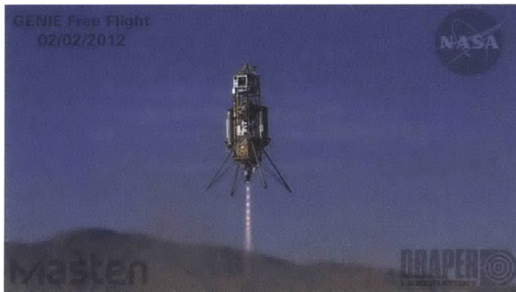
Figure 1-6: Draper’s GENIE System guides the Masten Xombie terrestrial rocket during a controlled hop. Image credit: Draper Laboratory
