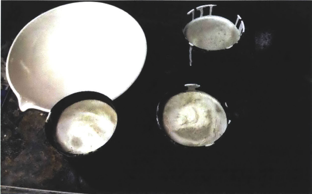
Figure 4.29: 3" Cylindrical plastic mold filled with gypsum mixture
