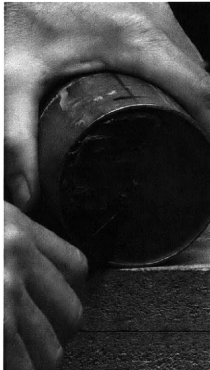
Figure 4.19: A straight edge is used to remove soil and debris from the surface to create a level and clean soil surface (Germaine and Germaine, 2009).
