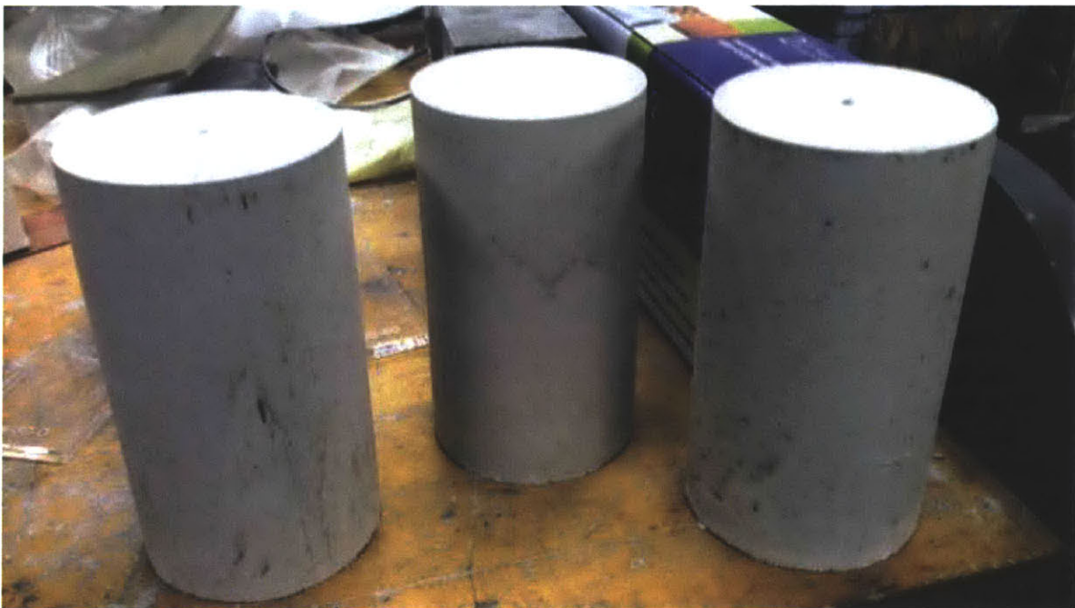
Figure 4.30: Cylindrical Gypsum specimens after drying and releasing from molds
