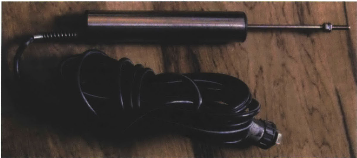
Figure 4.37: Trans Tek 2.5 cm LVDT
