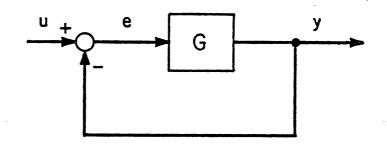
Figure 1. Basic MIMO Linear Feedback System
