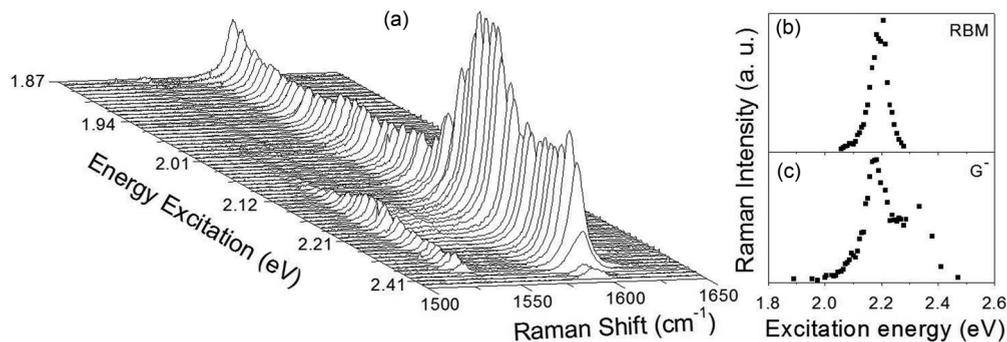
FIG. 2. The  $G$ -band spectra obtained with 70 different excitation energies. (b) Raman excitation profile (intensity versus laser energy) of the RBM peak at  $308\text{ cm}^{-1}$  associated with the (6,5) nanotube. (c) Raman excitation profile of the  $G^-$  peak at  $1528\text{ cm}^{-1}$ .
