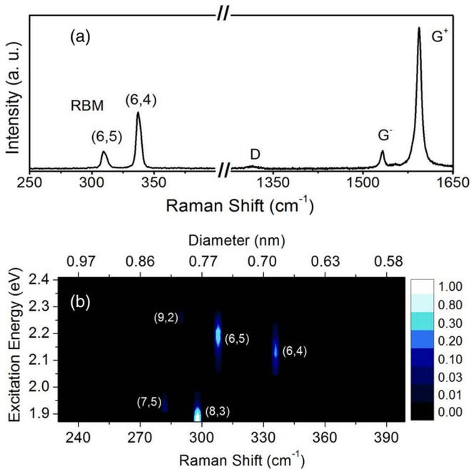
FIG. 1. (Color online) (a) Raman spectra sample recorded with the 585 nm (2.12 eV) laser line, showing the most important spectral features: RBM,  $D$ , and  $G$  bands. (b) Resonance Raman maps of RBM bands obtained with different excitation energies, revealing the existence of nanotubes with different chiralities in the sample.
