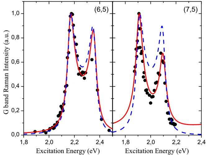
FIG. 3. (Color online)  $G$ -band REP for (6,5) and (7,5) carbon nanotubes. The black circles are experimental data and the full red line is the present calculation with all matrix elements, while the dashed blue line is the same calculation using constant matrix elements. The electronic gap between the valence and conduction bands was corrected in a few electronvolts to fit with the experimental transitions.
