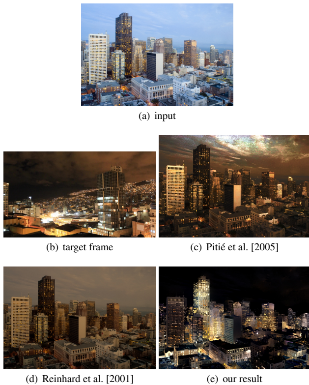
Figure 12: Global methods generate only moderately convincing results (c,d). In comparison, our local affine transforms provide more flexibility in modeling spatially varying color changes, which produces a better result (e).
