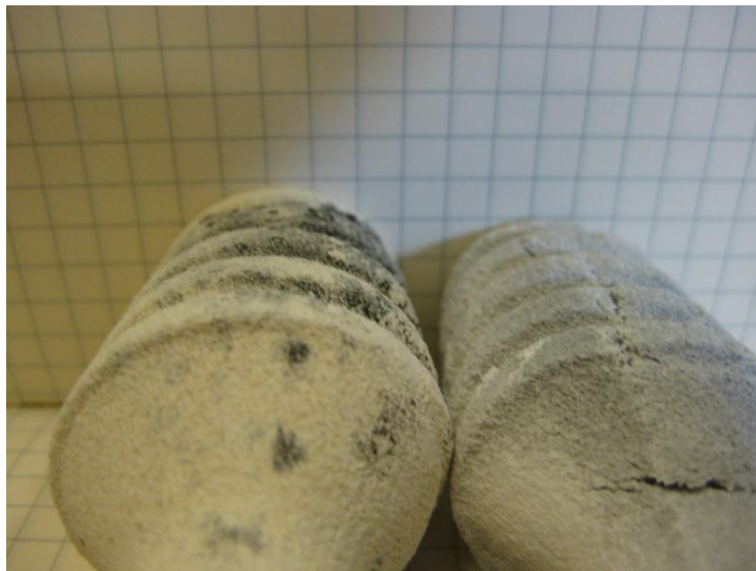
Figure 11: Comparison of a 403C sample (left) to a V18 sample (right), against quarter-inch graph paper (each square is 6.35mm tall). The V18 sample is significantly shorter and flatter than the 403C sample.
