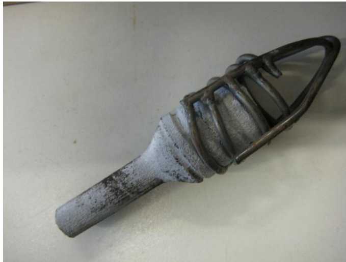
Figure 13: Double-reinforced tensile jig after high-temperature testing. The coils have separated to about twice their original pitch, no longer fitting the sample's threading (and becoming firmly stuck on the sample, in the process).
