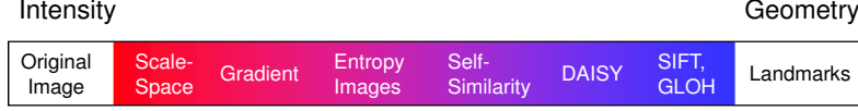
Figure 4. Continuum between feature- and intensity-based registration, augmented with exemplary approaches. Arranged by the uniqueness of descriptors.
