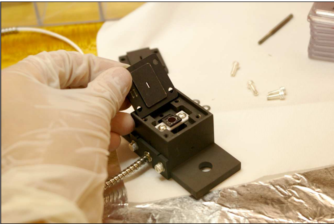
Photo 2 – Final assembly of the wall-mounted photodiode boxes on August 29, 2011.
