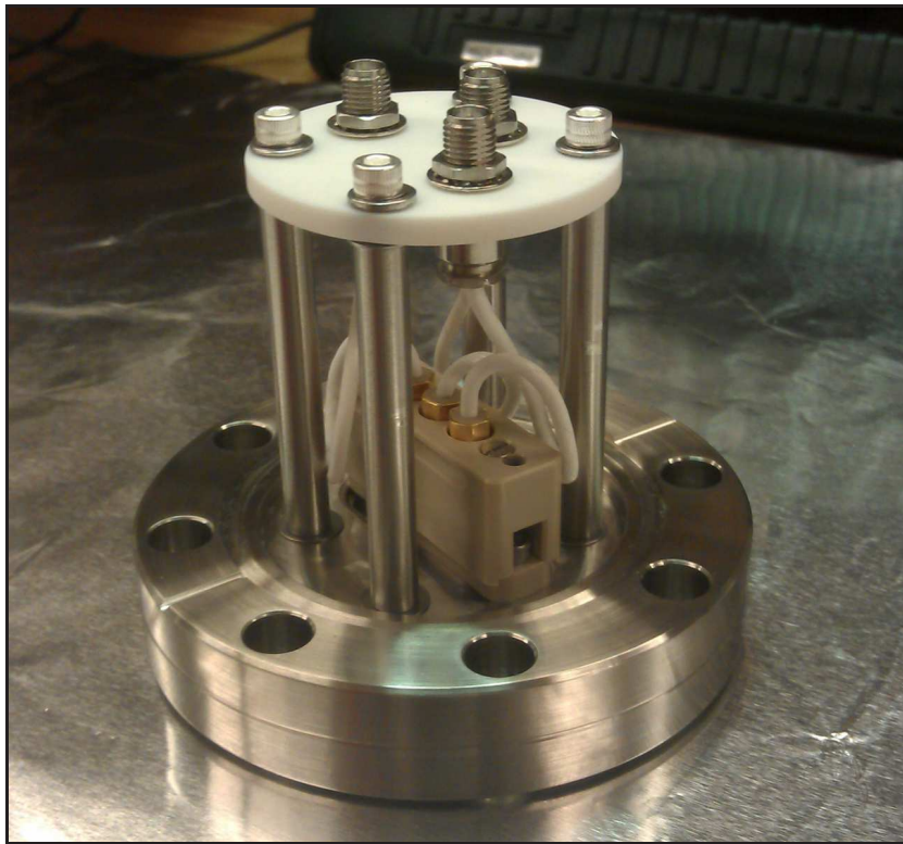
Photo 5 – Custom-built “triple PEEK” vacuum feedthrough to carry diode data out of Alcator C-Mod with fully coaxial signal path. Assembled and ready for installation, August 16, 2011. See Appendix F for manufacturing drawings for feedthrough.
