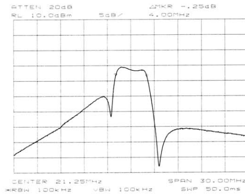
Figure 5-2: Measured frequency response of elliptical bandpass filter.
