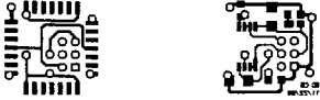
Figure A-1. Plots of fingertip printed circuit board copper layers, actual size. (a. Left) Top copper layer. (b. Right) Bottom copper layer.
