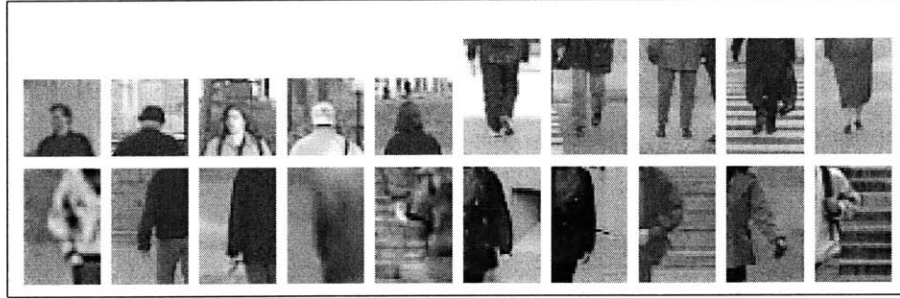
Figure 4-4: The top row shows examples of “heads and shoulders” and “lower bodies” of people that were used to train the respective component detectors. Similarly, the bottom row shows examples of “left arms” and “right arms” that were used for training purposes.
