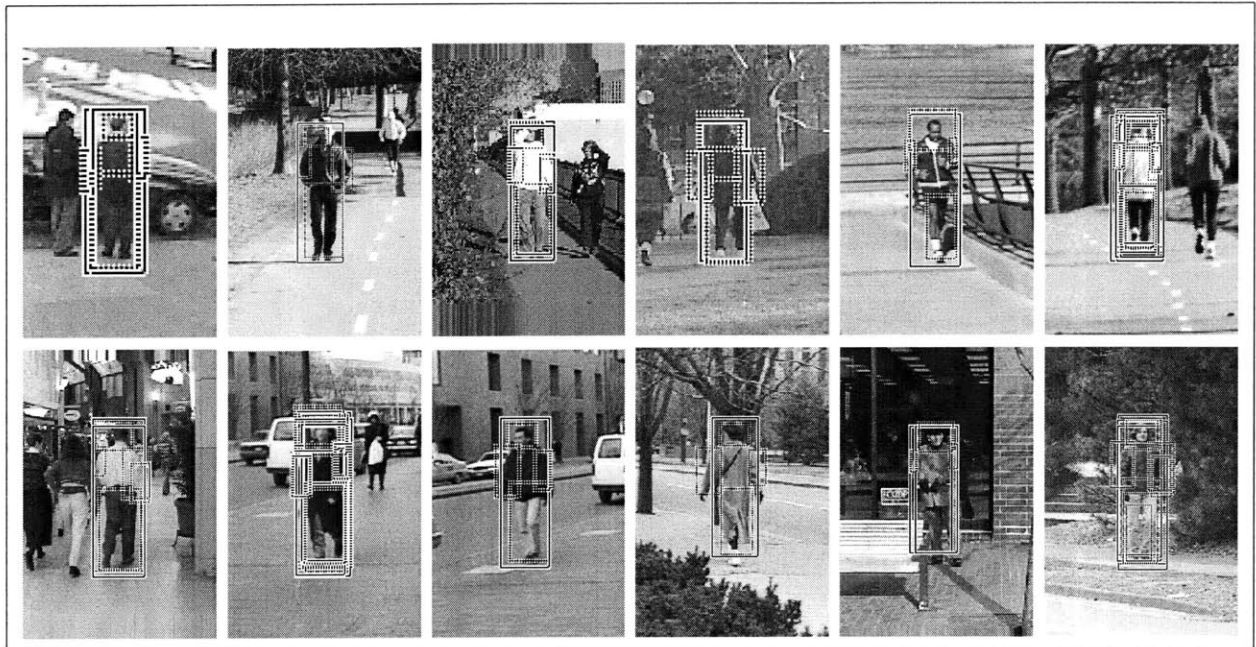
Figure 4-7: Samples from the test image database. These images demonstrate the capability of the system. It can detect running people, people who are slightly rotated, people whose body parts blend into the background (bottom row, second from right - person detected even though the legs are not), and people under varying lighting conditions (top row, second from left - one side of the face is light and the other dark).
