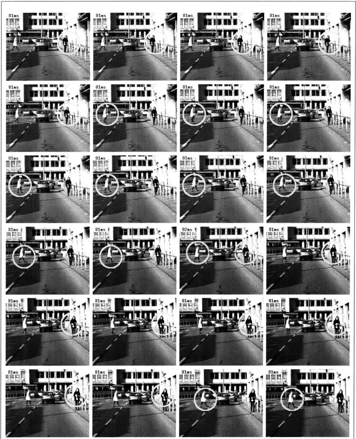
Figure 5-5: A sequence showing the single most salient location for each frame as processed by the system of [Itti et al. , 1998, Itti and Koch, 1999]. Our people detection system can use this focus of attention module as a preprocessor to target specific areas of an image.
