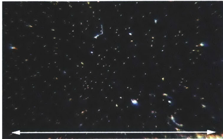
Figure 4.7: Excised bovine coronary embedded with fluorescent microspheres, expanded with a slotted tube stent, and photomicrographed under ultraviolet illumination. The arrow displays the distance between the proximal and distal tips of one stent cell measured along the longitudinal axis, 1.9 mm. The coronary tissue appears black, the beads fluoresce yellow, and the small white circles are holes in the tissue previously occupied by collateral vessels oriented normal to the coronary surface.
