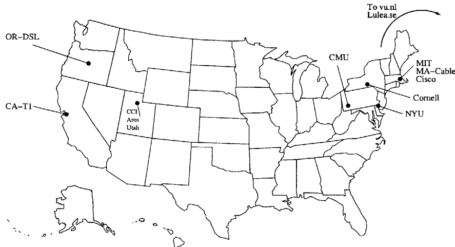
Figure 5-1: The current 13-node RON deployment. Five sites are at universities in the USA, two are European universities (not shown), two are “broadband” home Internet hosts, one is located at a US ISP, and three are at US corporations.
