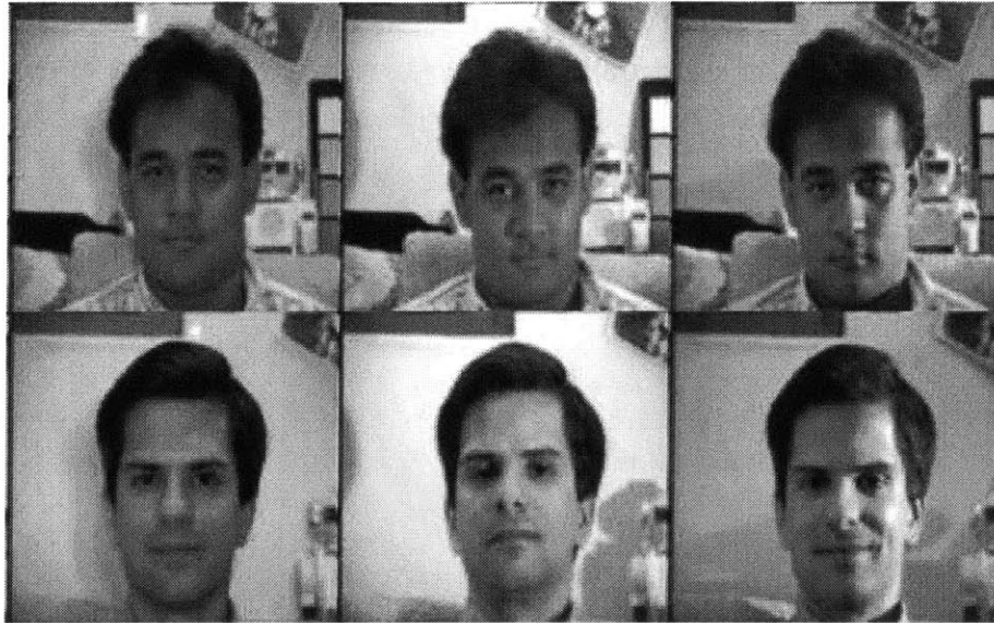
Figure 8-4: Six of the static test images from Turk & Pentland (1991) used to evaluate the ratio template face detector. Each face appears in the test set with three lighting conditions, head-on (left), from 45 degrees (center), and from 90 degrees (right). The ratio template correctly detected 71% of the faces in the database, including each of these faces except for the center image from the first row.
