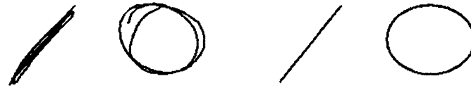
Figure 6-2: An overtraced oval and a line along with and the system's output.
