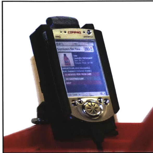
A close up view of the Voyager PSA Client—a wirelessly networked Pocket PC mounted to a shopping basket.
