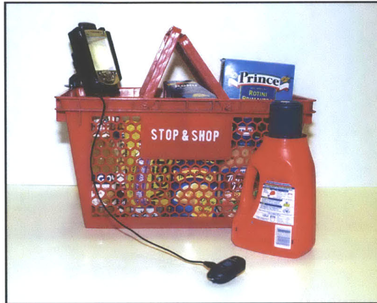
The Voyager PSA client consists of a Pocket PC PDA with an attached barcode scanner mounted to a plastic shopping basket.
