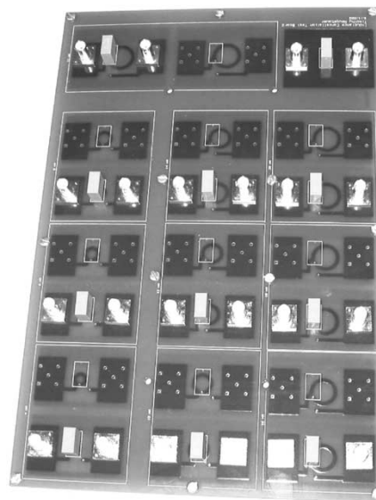
Fig. 8. Test comparison board. A capacitor without inductance cancellation is in the upper right corner. Every other layout has a transformer with a different shunt path inductance.
