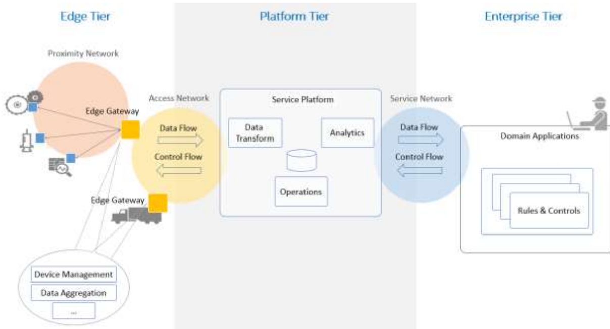
845 Figure 7-2 Three-tier IIS Architecture
