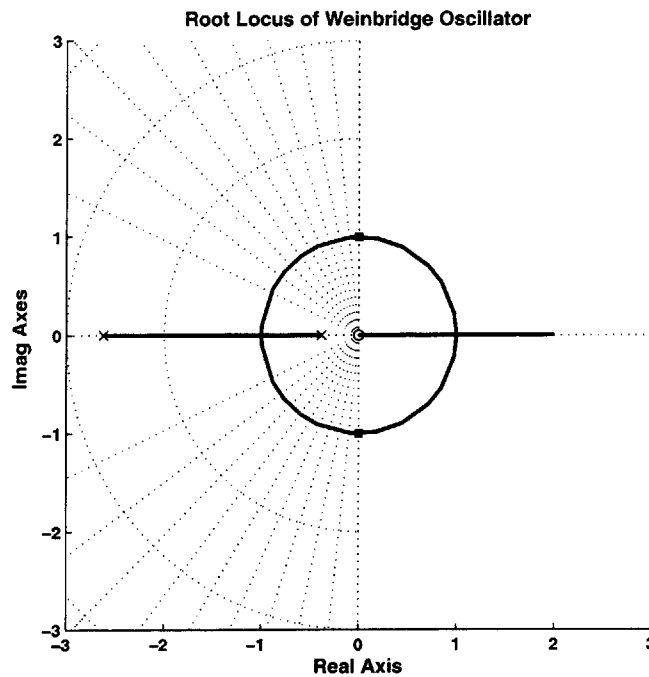
Figure 6-7: Root-locus of the two-pole system with zero at DC.
