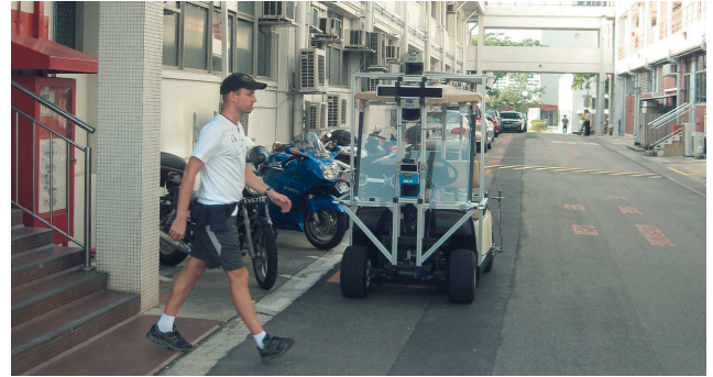
Figure 6—Carcel’s Outdoor Setup. A picture of the actual golf car route showing the pedestrian crosswalk that poses a hazardous blind-spot for the golf car. This setup makes visual confirmation of a pedestrian difficult before he is actually on the road.
