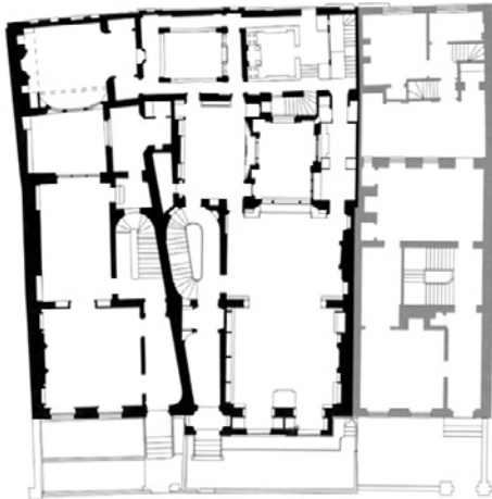
1822 Soane continues to renovate No. 12 & No. 13 Lincoln's Inn Fields refiguring the stair; adding the Monument Court- yard, Dressing Area, Study, New Break- fast Parlor, the start of the Colonnade; and renovating the Dining Room.
