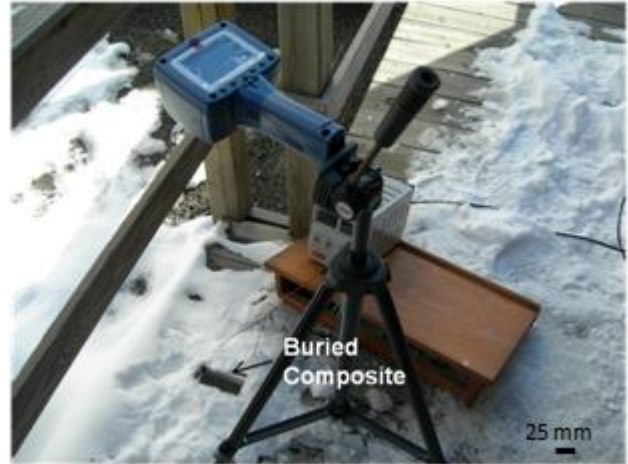
Fig.4. De-icing experimental setup of the heated (22.2W for 15min) composite material embedded in snow (-10°C, 2.5cm of snow thickness).
