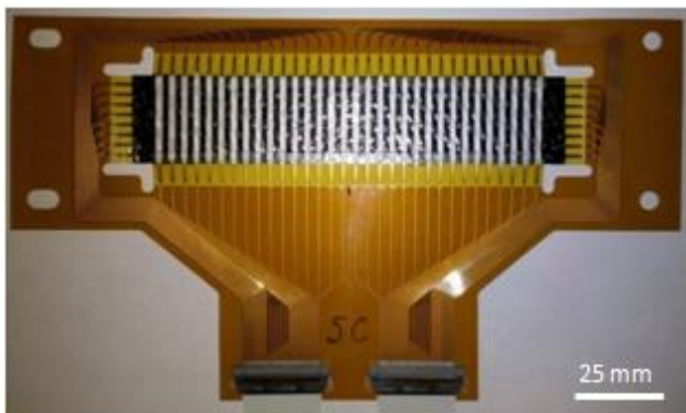
Fig. 1. Ice-detection sample. The electrodes (perpendicular white lines) were printed by direct writing.
