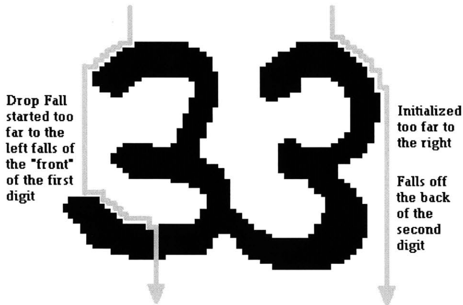
Figure 4.1: Bad starting points for Drop Fall Segmentation
