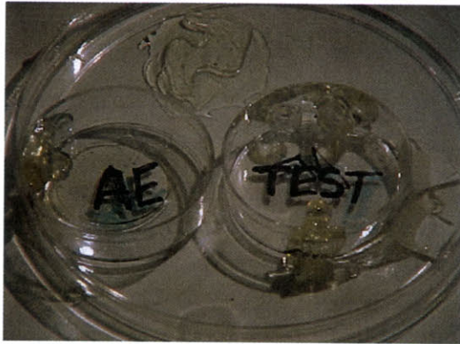
Figure 2-2: The chamber consisted of two dishes placed a distance of 1.15 mm from each other. The left dish contained AE, the reference fluid. The right dish contained one of the test solutions, K21, K43, K348 or K696. The gel straddled the two dishes such that each end of the gel dangled in one of the two baths.
